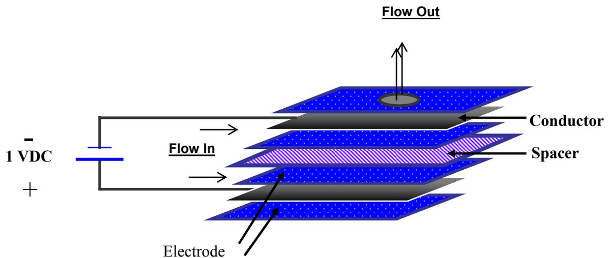
**Figure 9: Single Stage Process Flow Diagram**
